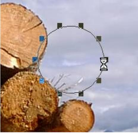
Figure 2. Appearance of an initial spline curve fitting tool. The spline control points can be moved about, merged or created, to fit a face. The whole pattern can also be dragged to a face.
